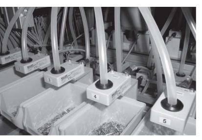
Ring sensors are used for feed control with screws, nails etc.
